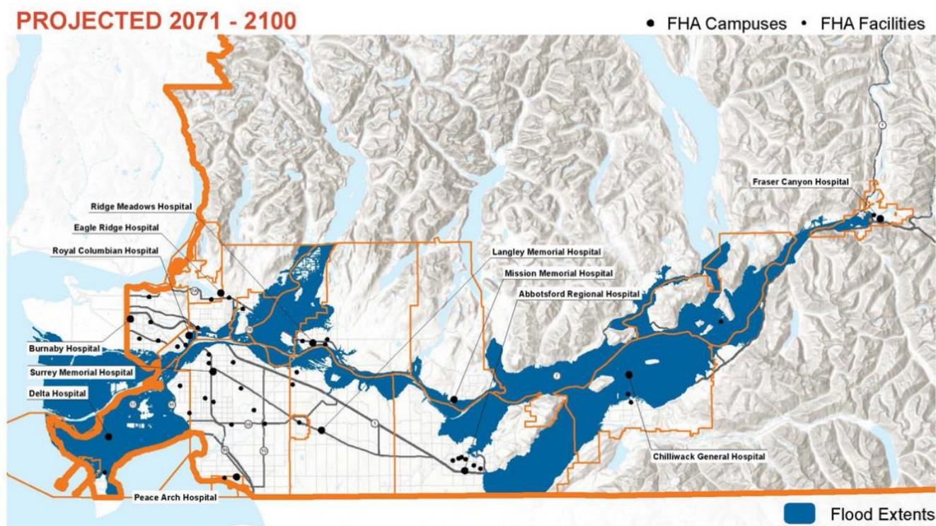
Figure 31: Floodplain projections and facility locations for FHA (Facilities Management, 2019)
