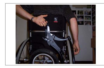
Setting up the perch for the free wheel which clamps to the rear rigidizer bar when not in use is simple enough but I suggest taking time to experiment with the angle the "U" shaped post is fixed at. It took me 15 to 20 seconds of fiddling each time I wanted to clamp the free wheel to the post. After I adjusted it so that the clamping shim was parallel to the straight surface when the free wheel hung from my finger it took less than 5 seconds and no fiddling.
